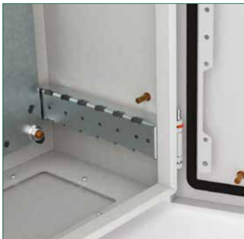
Wiring support, creation of an internal structure and depth adjustment of the accessories at 25 mm intervals thanks to the universal cross-pieces (with front fastening to the universal brackets).
